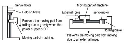
The brake has the following operation delay time. ON and OFF of the operation, please ensure the brake operation time.
