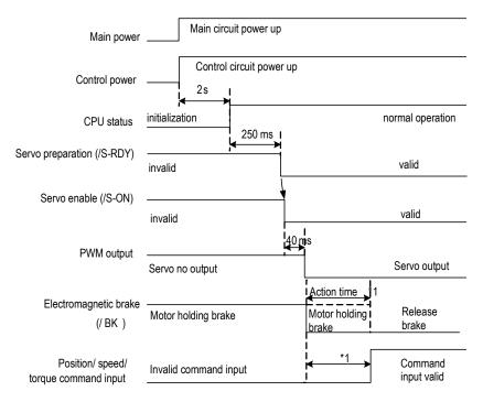
There is a delay in the electromagnetic brake operation. The operation time varies depending on the type of brake. It is recommended to be more than 100ms to ensure that the electromagnetic brake is completely released when the command is input. This time can be omitted when motor is not braked.
