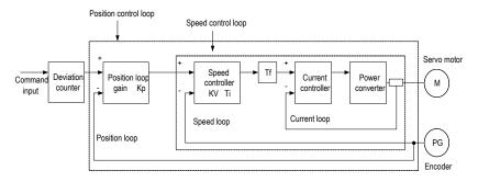
Please adjust each servo gain one by one after fully understanding the composition and characteristics of the servo units if the servo gain needs to be adjusted manually. In most cases, if one parameter changes significantly, the other parameters must be adjusted again. In order to confirm the response characteristics, preparations must be made to observe the output waveform of the analog monitor using a measuring instrument.
