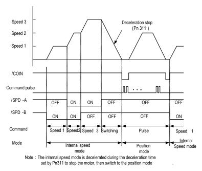
b) Digital input signal distribution mode is parameter configuration (Pn600=1 default parameter)
