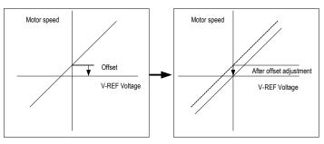
There are two methods of automatic adjustment and manual adjustment of offset adjustment. Automatic adjustment is automatic adjusting command offset (Fn100) and manual adjustment is manually adjusting command offset (Fn101). For details, see "Auxiliary Functions".
