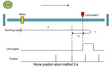
b.Start the home position return  $\rightarrow$  forward limit valid $\rightarrow$  search for the falling edge of forward limit at low speed reverse direction $\rightarrow$  search for Z pulse in reverse direction.
