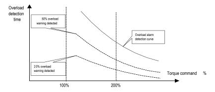
2. Change of the detection time of the overload warning (Er. 720)
