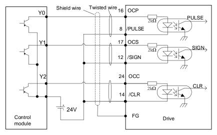
If the linear drive input port is used to receive the external 24 V collector open circuit input signal, connect a 2k resistor in series to limit the current in the circuit, otherwise, the linear drive input port will be damaged.
