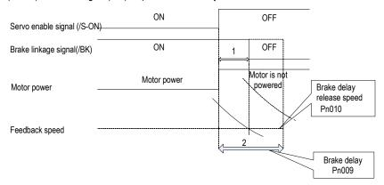
When the motor speed is lower than the set value of Pn010 after the power to the servo motor is
