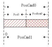
As shown in the figure above, the first position command setting value is PosCmd0. After the pulse of Pos0 is run, the operation ends and the remaining PosRem0 pulses are not completed. If the second absolute position command PosCmd1 is inserted at this time, the total number of pulses of the second position command operation is PosCmd1- Pos0. That is, the second absolute position value PosCmd1 is the absolute position 0 bit reference point, and the final running position value is PosCmd1.
