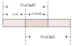
As shown in the figure above, the first position command setting value is PosCmd0. After the pulse of Pos0 is run, the operation ends and the remaining PosRem0 pulses are not completed. If the second relative position command PosCmd1 is inserted at this time, the total number of pulses of the second position command operation is PosCmd1. That is, the second relative position value
