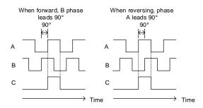
Parameter Pn072 can be set to revert the logic of the AB phase signal of the divided output pulse.
