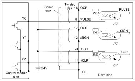
2.Control modules is PNP type (common anode):
