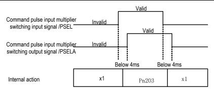
2. Command pulse input magnification switching wiring
