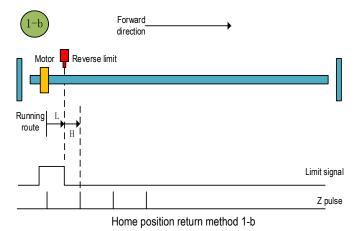
a.Start the home position return  $\rightarrow$  search for the forward limit at high speed forward direction  $\rightarrow$  encounter the forward limit rising edge  $\rightarrow$  decelerate to 0  $\rightarrow$  search for the falling edge of forward limit at low speed reverse direction  $\rightarrow$  search for Z pulse in reverse direction.
