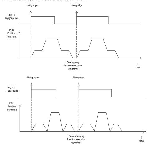
Note: When the overlap occurs, the previous instruction setting takes effect. When the previous instruction runs to the deceleration point, it runs the next instruction. Note: In speed mode, this bit indicates the speed command unit.
